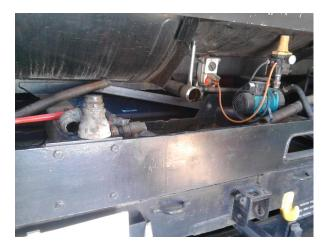
The output piping from the fresh water tank on the service wagon has also been receiving some attention.
