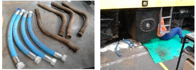
An "interesting" point about the thinking of NZR (as it was then) is that due to the size of the fittings, 1250psi hose has to be fitted, even though only 100psi pressure is required. The 1250psi hose is of course dearer than 100psi hose!
