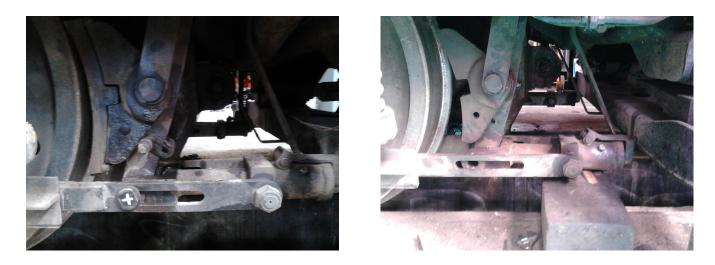
Further inspection has revealed that some of the other locating pins also need to be replaced.
